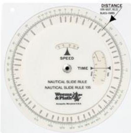
The **Nautical Slide Rule** quickly solves and speed-time-distance calculation and is a staple item for marine navigators today. By aligning the disks to any two known factors of an equation, the tool displays the unknown factor. Many of Captain Weems inventions were based upon this "computer" concept, such as is seen in this nautical adaptation of a slide rule - a tool common to all engineers prior to modern computers.
